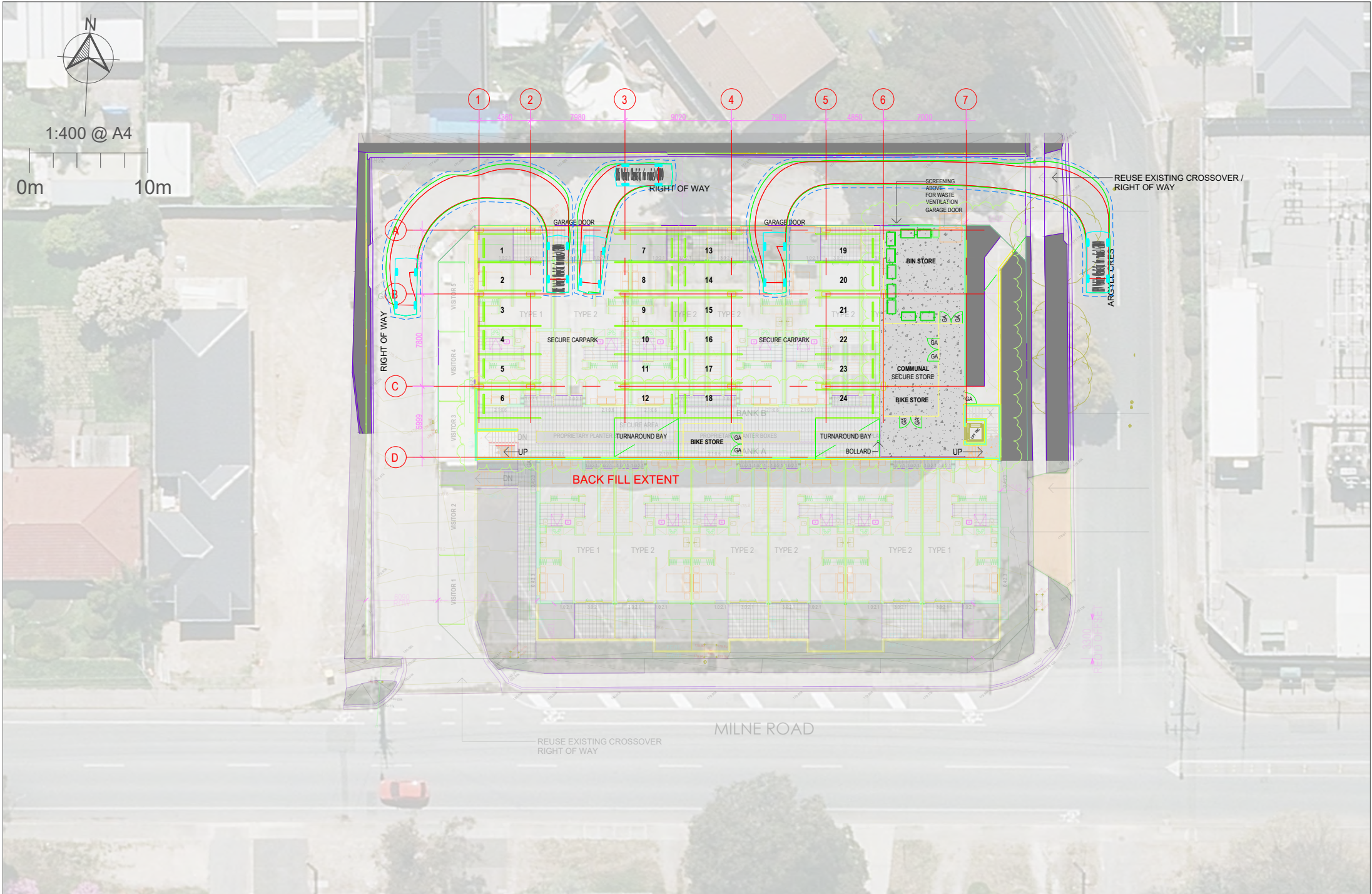
FIGURE 3: B99 ACCESS PAST INTERNAL WASTE COLLECTION VEHICLE INCLUDING EASTERN ROLLER DOOR ACCESS, AND SIMULTANEOUS B85 WESTERN ROLLER DOOR ACCESSIBILITY
