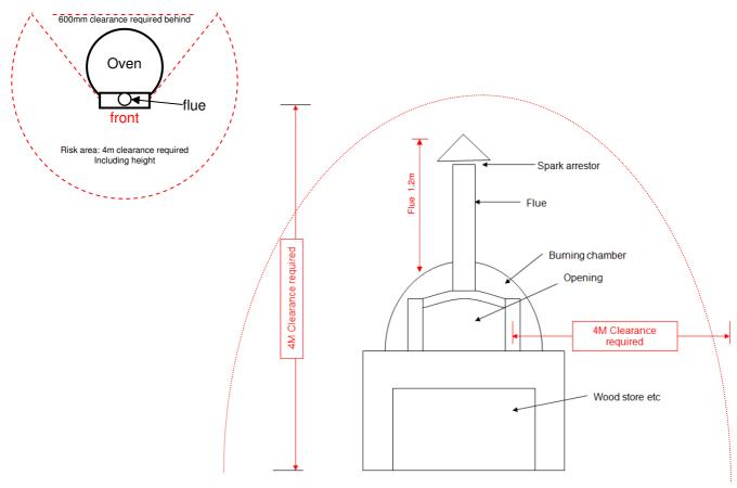
NOTE: The 4m clearance in height is from ground level and applies to a 180 degree arc surrounding the pizza oven.
